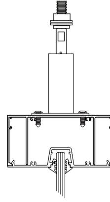
Seismic Pocket Headtrack
