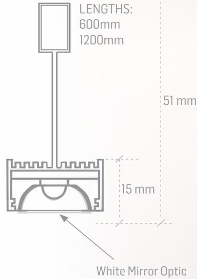
Gridlux is designed to be configured for any space, variable ceiling heights and working planes. Light levels are accommodated through the system driver outputs.
