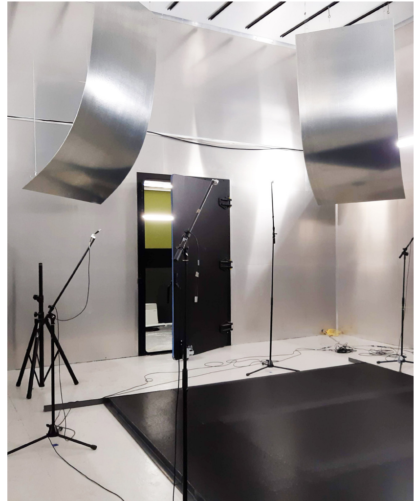
Figure 21. Reverberation Room at JSK Acoustic Testing Facility
