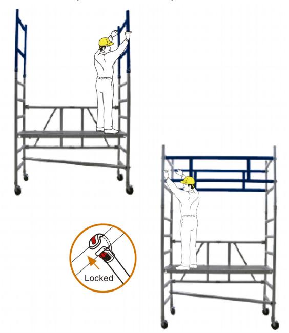
4. Erect the double horizontal brace. Clip it to the side of the guardrail with the gasper towards the outside. Clip the other end of the guardrail opposite. Make sure the scaffolding appears to be square. Ensure that it is fully locked. The frame should now be self-supporting.
