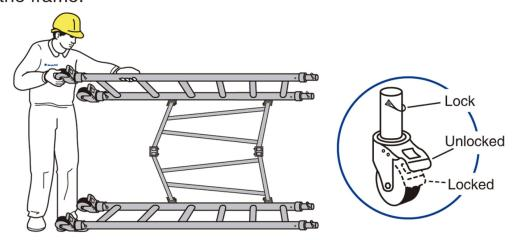
**2.**Open folded frame, lay it on the flat surface vertically, then lock four wheels and clip bottom brace onto frame. Then lay platform with hatch on the third rung of folded frame (count from bottom to top), lock it and inspect the stability of the whole structure.
