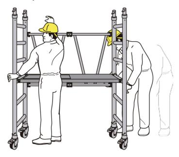
Note: All locking graspers should be primed before use, and released for dismantling or relocation.
